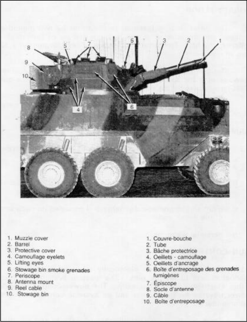
Figure 1-2-1 Turret Side View (Right-Hand Side)
